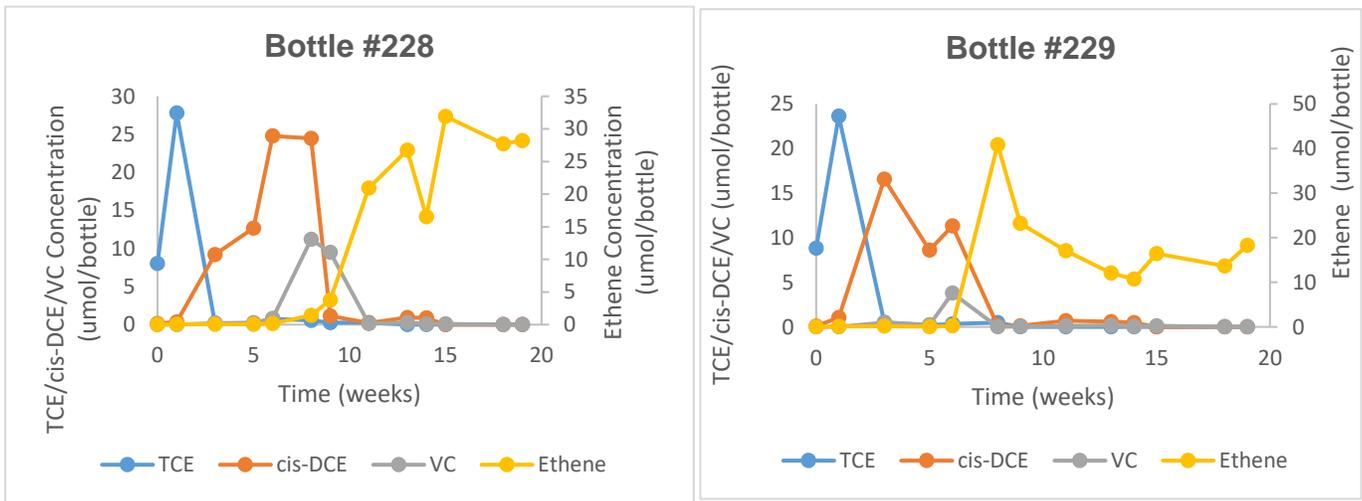
**Figure 4.** Effect of EVO (40 mM; 8,000 ppm) + SGO (250 mg/L) on TCE Degradation (19 weeks incubation time; n=2). Note scales and units.
