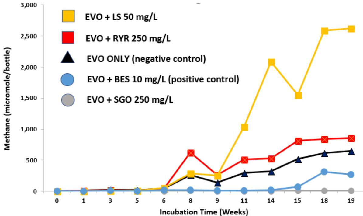
Conversely, both BES at 10 mg/L (**Figure 1** – blue circle) and Provect-CH4® SGO consisting of diallyl disulfide / diallyl trisulfide at 250 mg/L (**Figure 1** – grey circle) effectively reduced methanogenesis without having a negative effect on TCE catabolism (see below). Provect-CH4® EGO (natural garlic oil) exhibited results very similar to those obtained with the synthetic garlic oil, SGO (data not shown).
