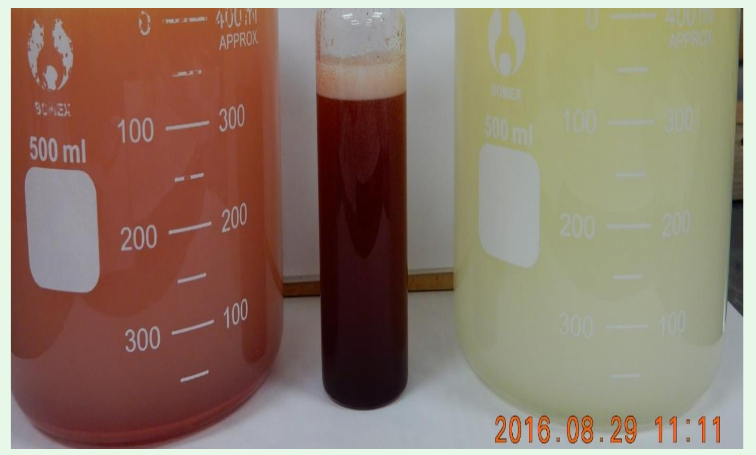
Photograph 1. Provect-ERD CH 4 ™ 15:1 Water:Oil (Left), 85% Carbon + 4% AMR Self-Emulsifiable Oil Concentrate (Middle), and 85% Carbon Self-Emulsifiable Oil Concentrate, no AMR (Right).
