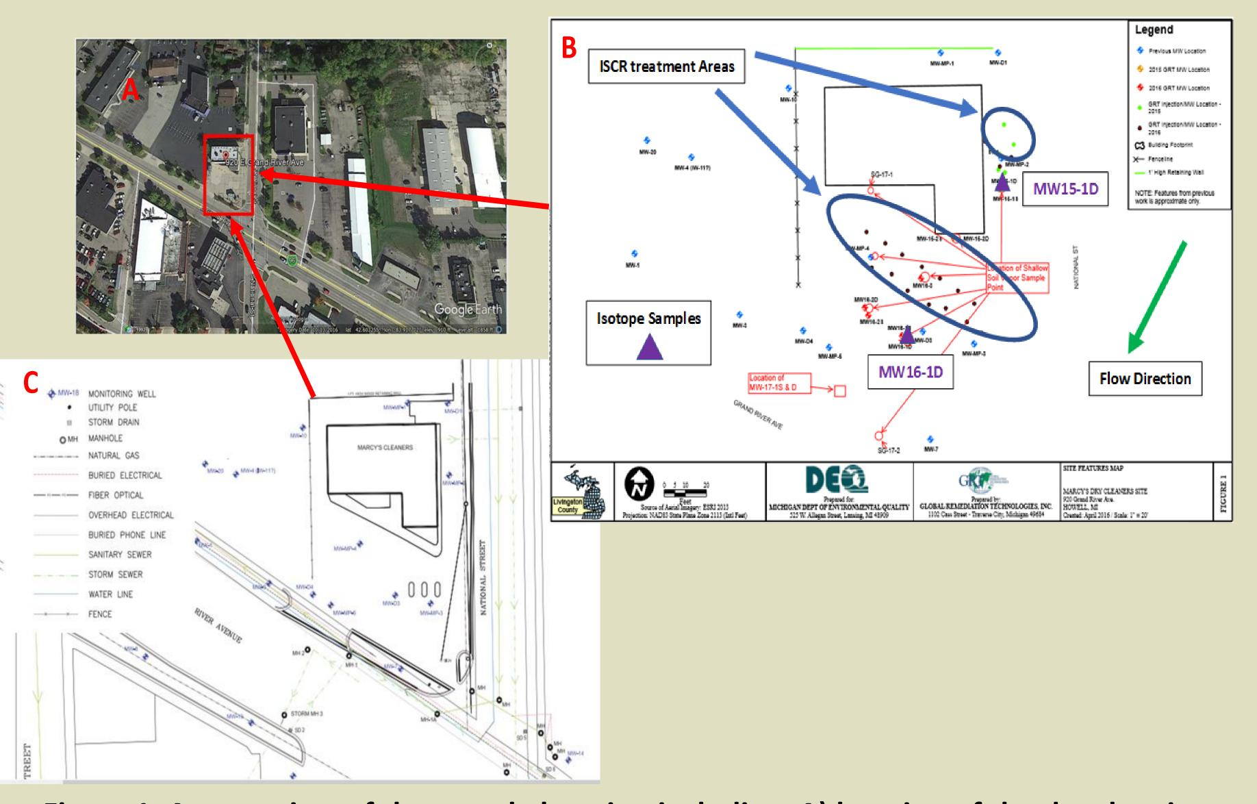
Figure 1: An overview of the sample location including; A) location of the dry cleaning facility; B) location of the monitoring wells including the sample wells reviewed in this study (purple triangles); C) distribution of sewer lines, storm water drains and utilities below ground in the study area.
