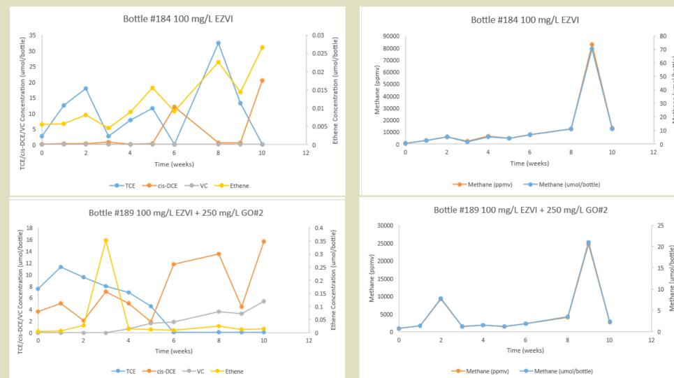
EZVI bench test data for contaminated soils with addition of TCE. The top graphs show results using EZVI with no AMR. The bottom graphs show results with AMR (Provect-CH4 EO).
