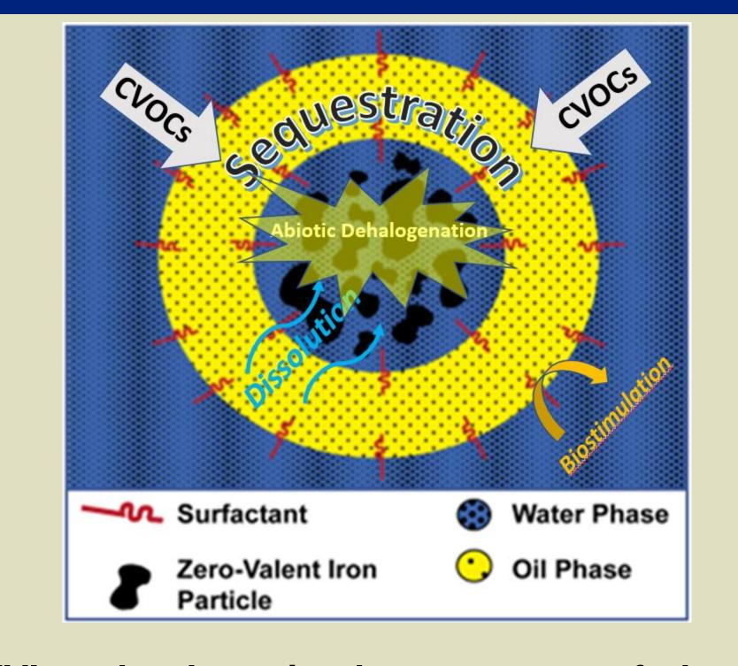
The key innovation surrounding the EZVI technology is the structure of the emulsion (Quinn et al., 2005). In order for the NASA patented technology to perform as designed, the emulsion structure, which is a water-in-oil type emulsification, is critical. The structure of the EZVI technology enables DNAPL treatment to proceed via 3 primary steps;
