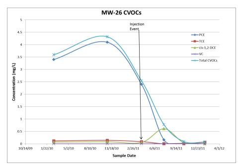
**Figure 2.** Concentrations (mg/L) in Groundwater vs. Time at MW-26 before and after in-situ injection event
