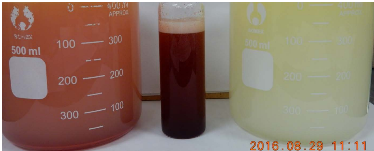
Photograph 1. Provect-ERD CH4™ 15: 1 Water:Oil (Left), 85% Carbon + 4% AMR Self-Emulsifiable Oil Concentrate (Middle), and 85% Carbon Self-Emulsifiable Oil Concentrate, no AMR (Right).
