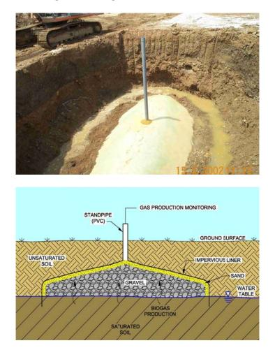
Figure 4. Large Scale In-Situ Test Cell
