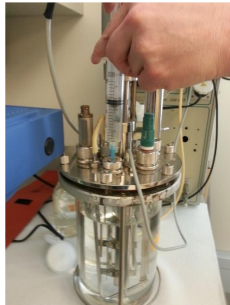
Figure 2. Close up showing biogas being collected with a syringe to monitor
