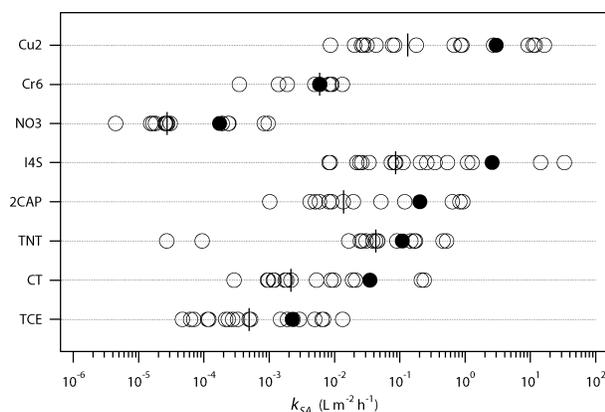
FIGURE 2. Dot plot of all rate constants ( $k_{SA}$ ) plotted versus reductate (ordinate). Open circles represent individual experiments; solid circles represent arithmetic mean, and vertical bars represent the median of individual values for each reductate. Data for the mean and median values are given in Table 1.
