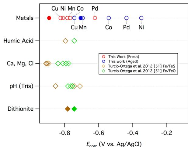
**Figure 4.** Summary of  $E_{corr}$  vs composition of the particles and the medium. (O) Effects of metal amendments (this study). (◇) Effects of solution composition.<sup>51</sup> Solid symbols are controls: (●) without metal amendments and (◆) in DI water. All data from Turcio-Ortega et al.<sup>51</sup> are without aging.
