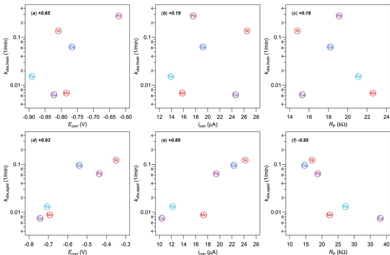
**Figure 5.** Correlations between electrochemical corrosion parameters and  $\log k_{\text{obs}}$  for (top row) fresh Fe/FeS and (bottom row) aged Fe/FeS. Correlation coefficients are given in italics. Rate constants from Table S2 and descriptor data from Table S3.
