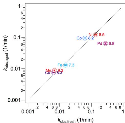
**Figure 3.** Plot of  $k_{obs}$  values for fresh particles vs those for aged particles. Data from Table S1. Dashed line is 1:1. Error bars, based on SD from fitting first-order kinetics, are shown but are smaller than the markers. Absolute hardness (from ref 66) is given as labels.
