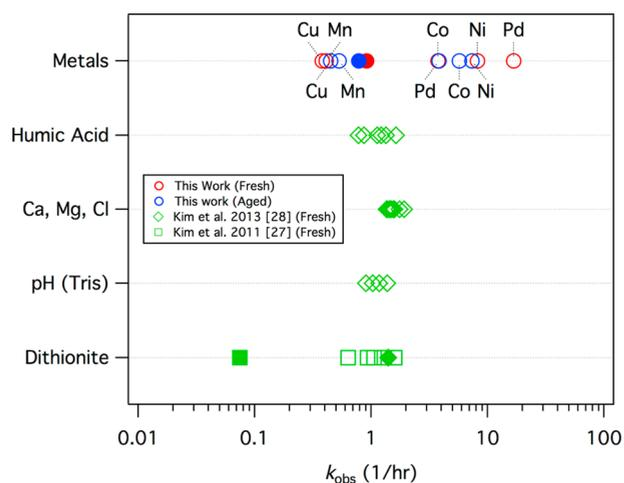
**Figure 2.** Summary of  $k_{obs}$  for TCE reduction by Fe/FeS vs composition of the particles and the medium. (○) Effects of metal amendments (this study). (◇) Effects of solution composition.<sup>28</sup> (◐) Effect of dithionite dose during synthesis.<sup>27</sup> Solid symbols are controls: (●) without metal amendments, (◆) in DI water, and (■) without dithionite.
