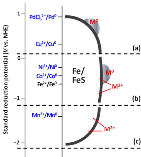
**Figure 1.** Conceptual model for metal interactions with Fe/FeS. Based on the classification scheme described in Li and Zhang<sup>30</sup> and standard reduction potentials for pH 7 from Pourbaix.<sup>37</sup>
