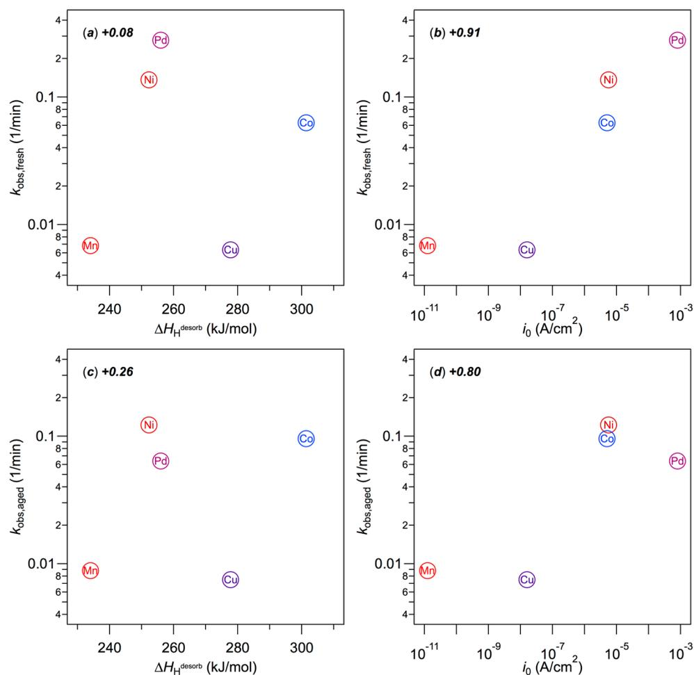
**Figure 6.** Correlations between hydrogenation-related parameters and log  $k_{\text{obs}}$  for (top row) fresh Fe/FeS and (bottom row) aged Fe/FeS. Correlation coefficients are given in italics. Rate constants from Table S1 and descriptor data from Table S3.
