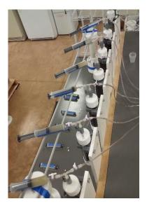
estimated average seepage velocity of 42 cm/day (1.4 ft/day) within potential ranges between 33 and 150 cm/day, or 1.1 to >5 ft/day under aquifer conditions). At predefined intervals (Time 0, 2, 4, 6 and 8 weeks), samples of column influent and effluent were analyzed for COIs, Fe/Mn RCRA metals, DO/ORP and pH. Production of methane was not monitored.
