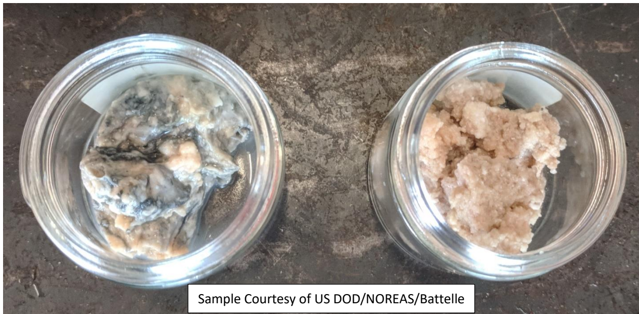
Photograph 1: EVO Scum (left) and EVO Crud (right) recovered from EVO-Treated Injection well, Six years after Initial EVO applications.
