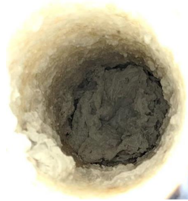
Photograph 1: EVO Scum (left) and EVO Crud (right) recovered from EVO-Treated Injection well, Six years after Initial EVO applications.
