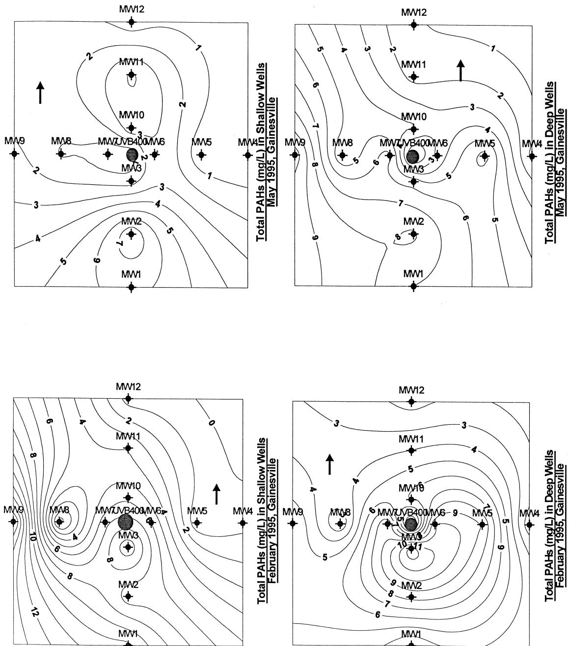
Fig. 4. Contour plots of Total PAH concentrations in groundwaters collected from shallow (3.7 m) and deep (6.1 m) ports at the Gainesville site on February 6, 1995 and May 31, 1995.
