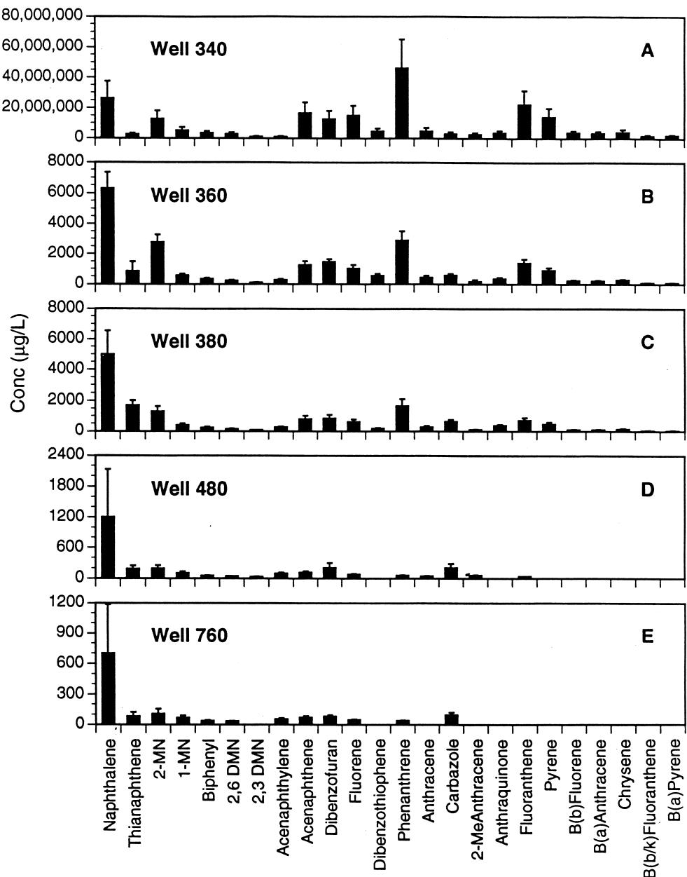
Fig. 3. Concentrations of PAHs in groundwaters collected from ACW Wells on September 9, 1994. The panels (A through E) are in order of increasing distance from the source of contamination. Error bars represent the standard deviation of triplicate samples. Note the changes in scale on the concentrations axes. The PAH compounds are listed in the order that they elute from the GC column.
