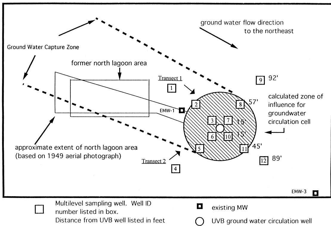
Fig. 1. Locations of sampling wells at the Cabot Carbon/Koppers facility in Gainesville, FL.
