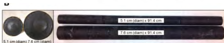
Figure 2. (A) Field plot of the permeable reactive barrier of SRPCs and monitoring wells; each SRPC location received five candles stack on top of each other; and (B) photograph of permanganate candles.
