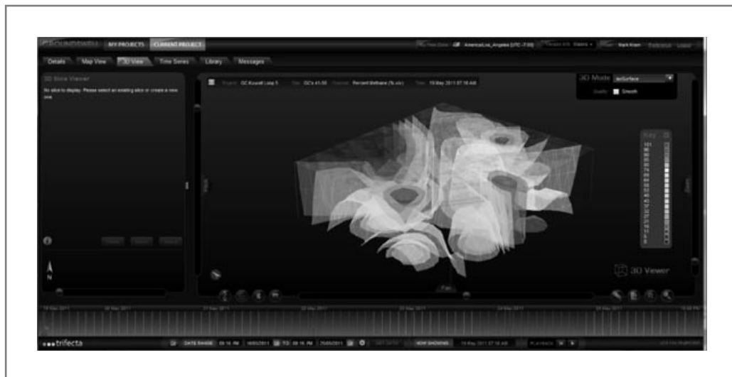
Exhibit 5. Time-stamped three-dimensional methane distribution underlying an air photo of a residential neighborhood
