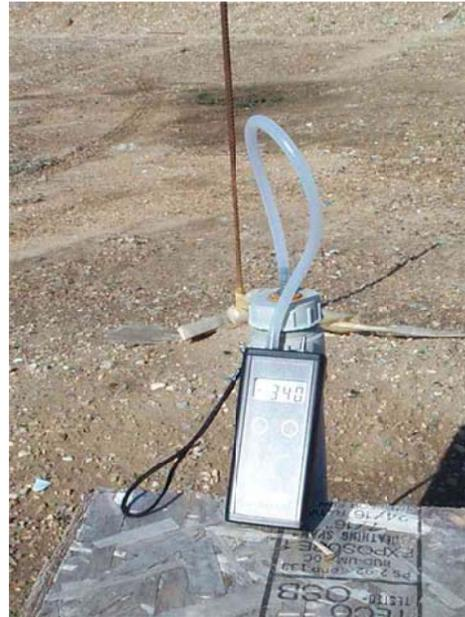
not unknown phenomenon. Continuous  $\Delta P$  measurements can document such variability. Continuous  $\Delta P$  has been routinely measured for sub-slab depressurization systems (SSDS), using such devices as Engineering Solutions Omniguard 4 Differential Pressure recorders.<sup>6</sup>
