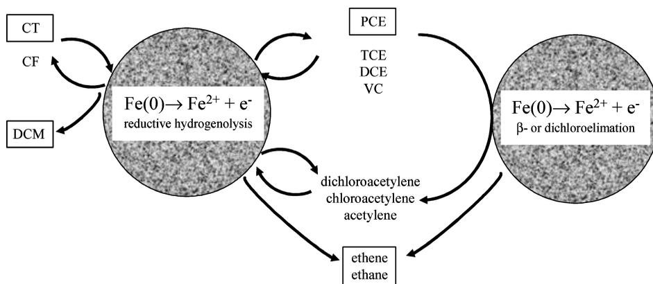
**Figure 2.** Dechlorination of chloromethanes and chloroethenes by ZVI; Fe(0).
