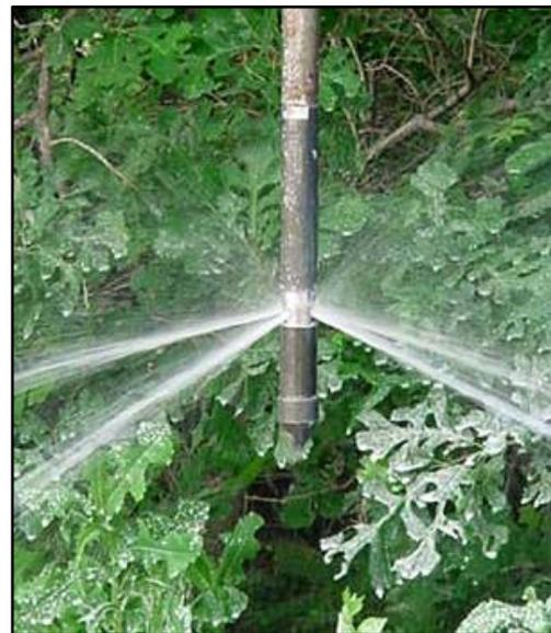
Tooling. Experienced drillers will have sufficient rod length on site to allow 3 to 5 injection points to be capped overnight to allow pressure to dissipate. This can help prevent backflow and surfacing of slurry as the injection rods are retracted. Likewise, experienced drillers will have on hand a variety of injection tips, some that direct the slurry horizontally (see for example GeoProbe's pressure activated tip).
